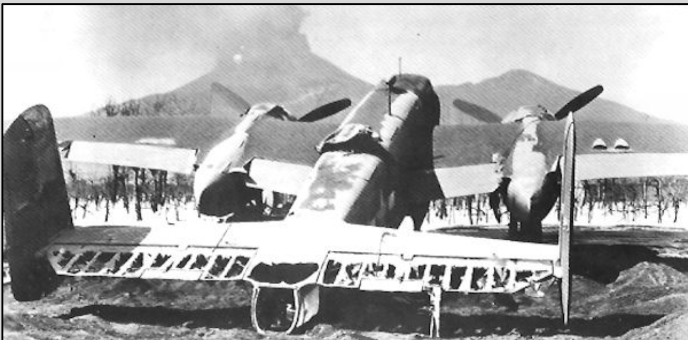
An unidentified B-25C Mitchell of the 340 th Bombardment group damaged after 18 th March 1944 Mount Vesuvius eruption at Pompeii Airfield, Italy. The volcano erupted, showering nearby airfields with tons of hot volcanic ash and brimstone and severely damaged a significant number of Allied aircraft. Aside from losing many of its B-25s, the group also suffered significant damage to its maintenance and accommodation facilities. (USAAF Photograph)
